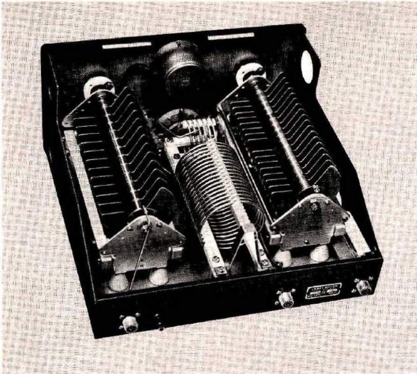
Typical antenna tuner construction. This is the popular Transmatch circuit described by W1ICP in QST . Many manufacturers build similar units around the same basic design, and many amateurs have built their own (photo courtesy the James Millen Company).
